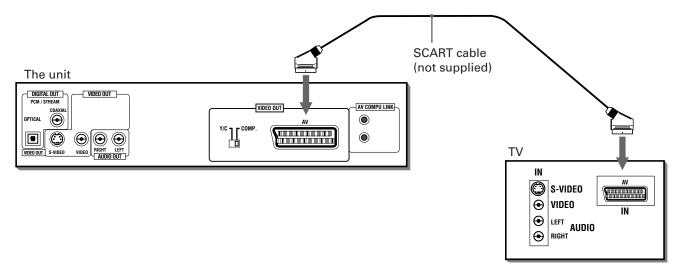
Set the COMP-Y/C switch correctly according to your TV.
